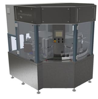
Semiautomatic technological solution intended to produce hot-cast leads in metal molds and subsequent assembly with the body - pencils. The machinery is equipped with a 50-position rotary table and metal molds, optimized for handling hot-cast leads. The molds are equipped with an integrated liquid thermal exchange system for efficient temperature regulation during production.
