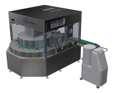
Automatic technological solution intended for producing poured stick. The machinery is equipped with a 50-position rotary table and metal moulds, optimized for handling hot pours of various stick materials, featuring an integrated liquid thermal exchange system for efficient temperature regulation during production.
