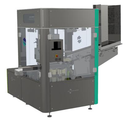
Automatic technological solution intended for filling-sealing tubes composed of different material. Machinery is designed to handle tubes characterized by versatility of use, both in make-up and for the treatment of different areas of the body (skin, hair and oral care).
