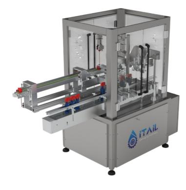
Technological solution for cap closure, featuring an automatic "Pick&Place" system that efficiently picks and places caps directly from the infeed conveyor. The filling and capping machines are also available in a monoblock configuration for streamlined integration.
