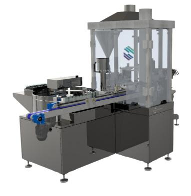
Automatic or semi-automatic technological solution intended for filling glass bottles and designed to manage the complete assembly of brush, dispenser, cap, dropper of liquid and/or low-viscosity mixtures.
