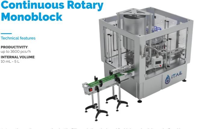
Automatic, continuous-motion bottle filling solution, designed for high productivity and offered in a monoblock configuration for both filling and capping, with adjustable heads to accommodate varying production speeds. It is suitable for liquid, dense, and semi-dense products, and the filler and capper modules are also available as standalone units.
