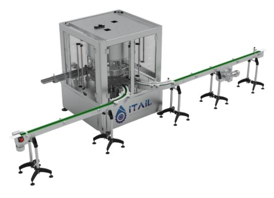
Automatic rotary solution with intermittent motion and an advanced nozzle tracking system, ideal for filling and capping plastic and glass bottles and jars containing liquid, dense, and semi-dense products across a broad viscosity spectrum. Both the filler and capper can also be configured asstandalone units.
