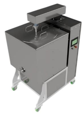
Heated Melter with Band Electric Heaters designed to keep the product agitated with four-zone independent temperature control, up to a maximum temperature of 120°C.
