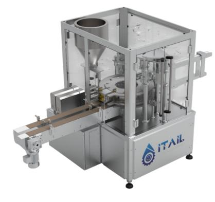
Automatic rotary solution with intermittent motion, designed for the filling and capping of plastic and glass bottles and jars, handling liquid, dense, and semi-dense products across a wide viscosity range. Both the filler and capper are also available as standalone units.
